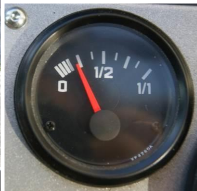
Water level gauche in cab
