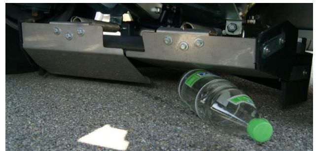
Coarse dirt flap (Boschung patent)
